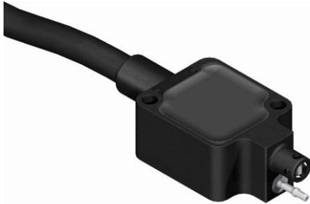
The gain, offset and thermal drift of the pressure sensor is digitally compensated to minimise errors and to create a single-ended, amplified output in the 0 to 5 Volt range. The output voltage changes with the absolute pressure applied to the pressure port.
